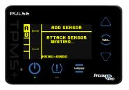
Attach a Sensor to the highlighted location's valve stem, and wait for a reading to populate. This may take up to 60 seconds.
